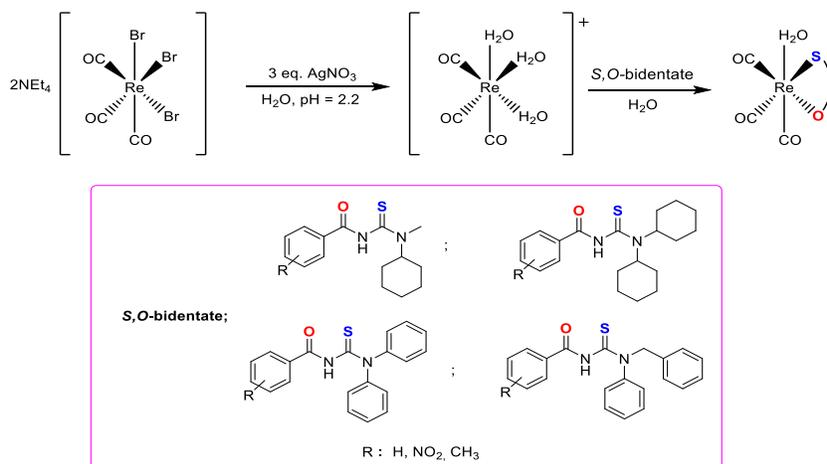
**Figure 1:** Schematic illustrations of various *S,O*-bid ligands and the synthesis of Re(I) tricarbonyl complexes
